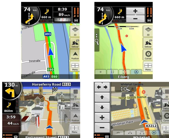
During navigation, the screen shows route information and trip data (left screenshot), but when you tap the map, additional buttons and controls appear for a few seconds (right screenshot). Most parts of the screen behave as buttons.
