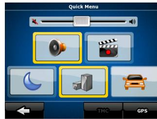
If you tap any of the switches in the Quick menu except for the Vehicle type, the Map screen immediately returns. A switch is on if its lamp is lit. The Vehicle type button is different. It is a multi-value button. It opens a list of available choices, and the symbol of the selected vehicle is shown on the button.
