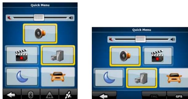
If you tap any of the switches in the Quick menu except for the Vehicle type, the Map screen immediately returns. A switch is on if its lamp is lit. The Vehicle type button is different. It is a
