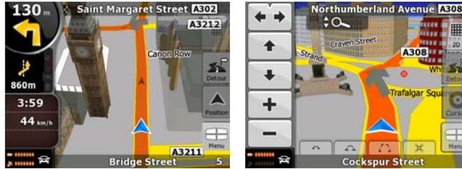
During navigation, the screen shows route information and trip data (left screenshot), but when you tap the map, additional buttons and controls appear for a few seconds (right screenshot). Most parts of the screen behave as buttons.
